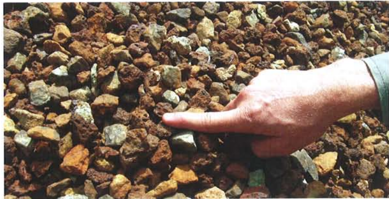
FIGURE 3 Gravel used as the infill in the geocell
